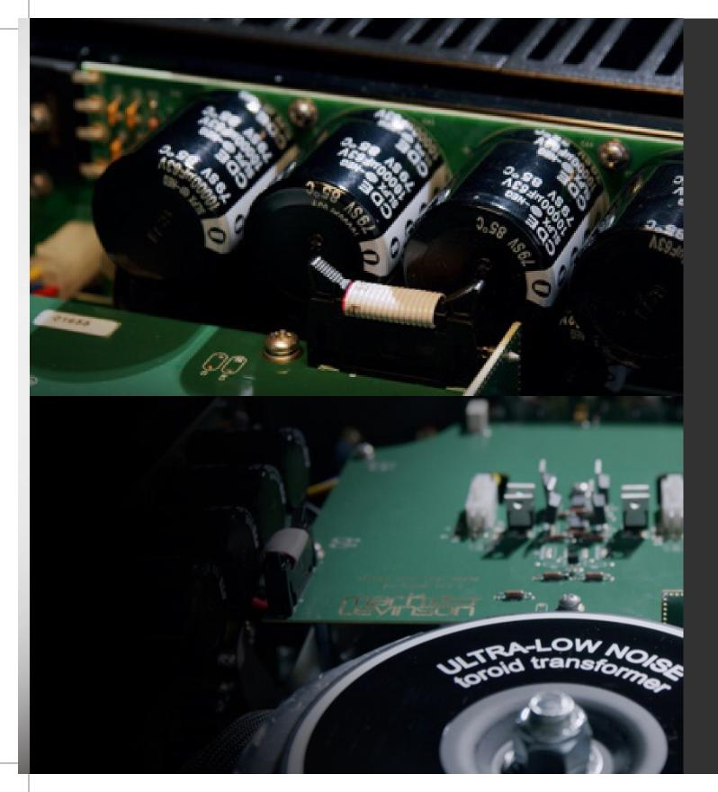
Four 10,000-microfarad capacitors per channel, located directly on the output stage circuit board, easily provide enough current for a conservative 135 watts per channel into 8 ohms, 270 watts per channel into 4 ohms, and 550 watts bridged in mono and stable operation into 2 ohms.
